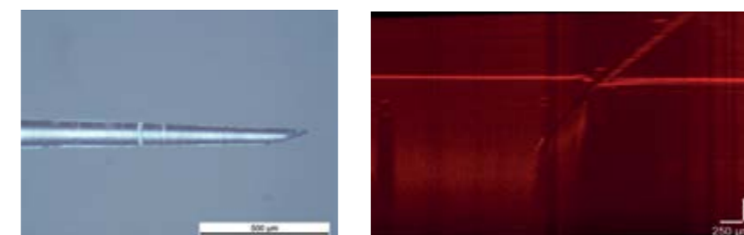
Above left: microneedle manufactured by laser machining; Above right: Microneedle inserted into tissue phantom.
