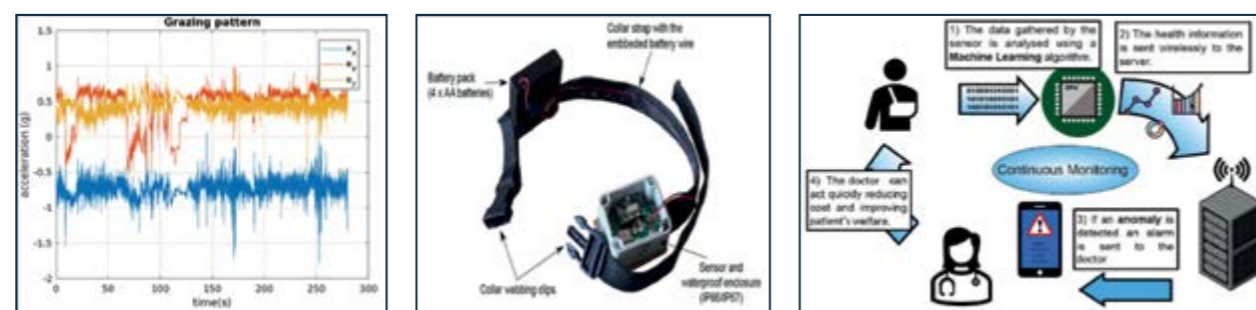
Figures Left: Results obtained for the detection of the grazing pattern of a sheep using the 3-axis accelerometer sensor (only) system. Middle: Early version of the sensor system prototype for the sheep (collar configuration). Right: A LoRaWan based model for patient activity monitoring.
