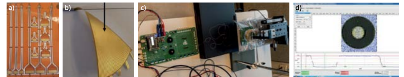
Figures from left to right: a) Flexible substrate with metal tracks, b) flexible substrate with transducer inserted into epidural needle, c) testing of the 64-element transducer using electronic circuitry, d) Successful picosecond laser machining of a 295 mm thick silicon substrate.
